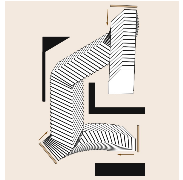
Stable Pushes to manoeuvre an object around obstacles. Adopted from Chapter 37, Fig 37.11 in Springer Handbook of Robotics.
