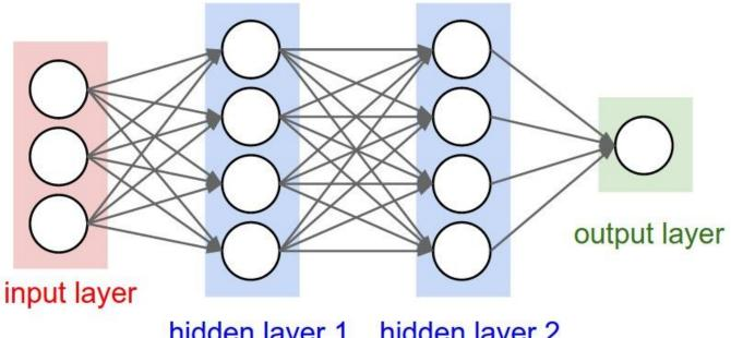
$h_1 = f_1(xW_1 + b_1)$   $h_2 = f_2(h_1W_2 + b_2)$  $y = f_3(h_2W_3 + b_3)$
