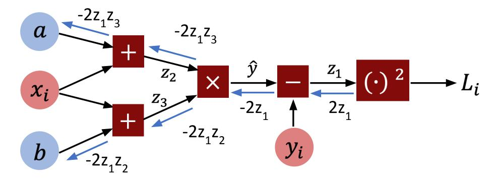
How many operations in the forward and backward passes? 5 in a Forward Pass, 4 in Backward
