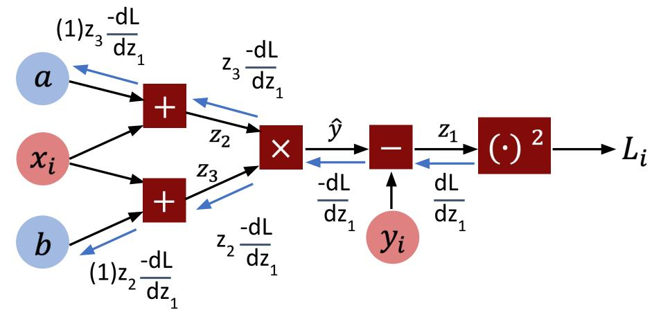
Backpropagation allows for sharing values in computation, increasing efficiency
